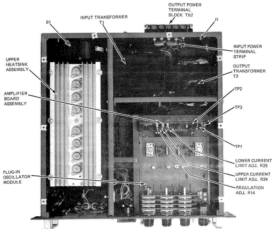
Figure 5-1. Model 501A Top View
