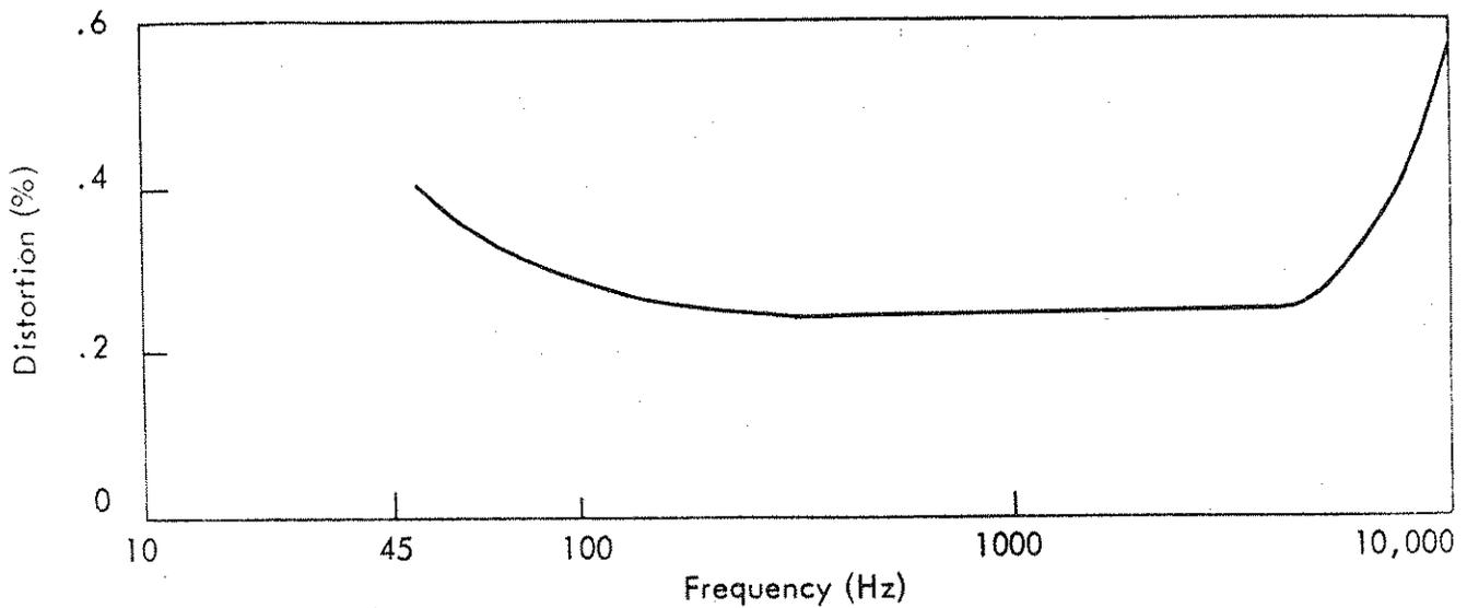
Figure 1-2. Typical Harmonic Distortion at Rated Power
