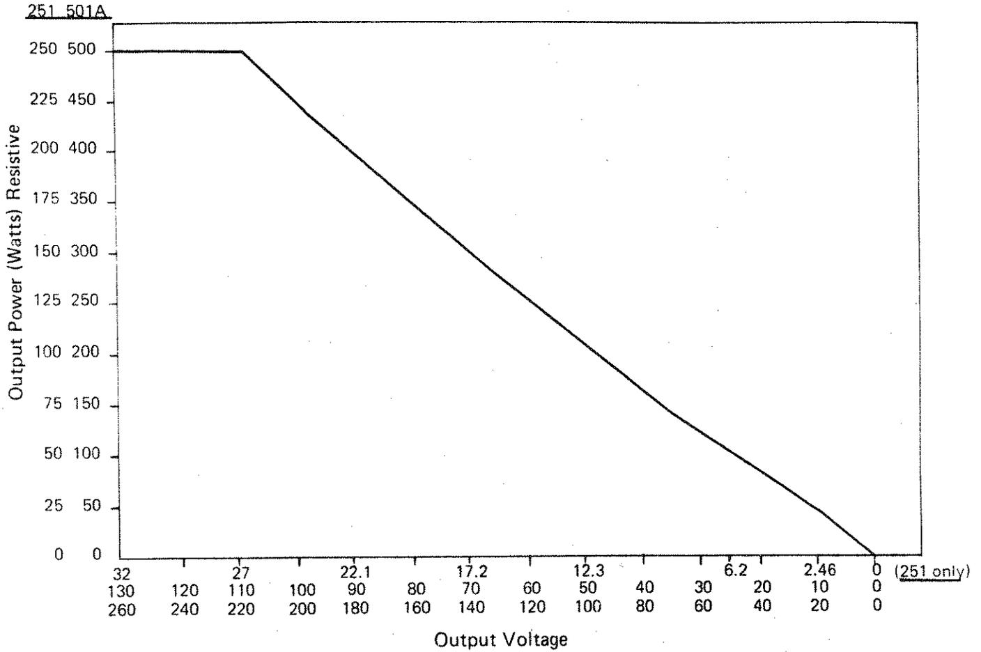
Figure 1-1. Power Output Derating
