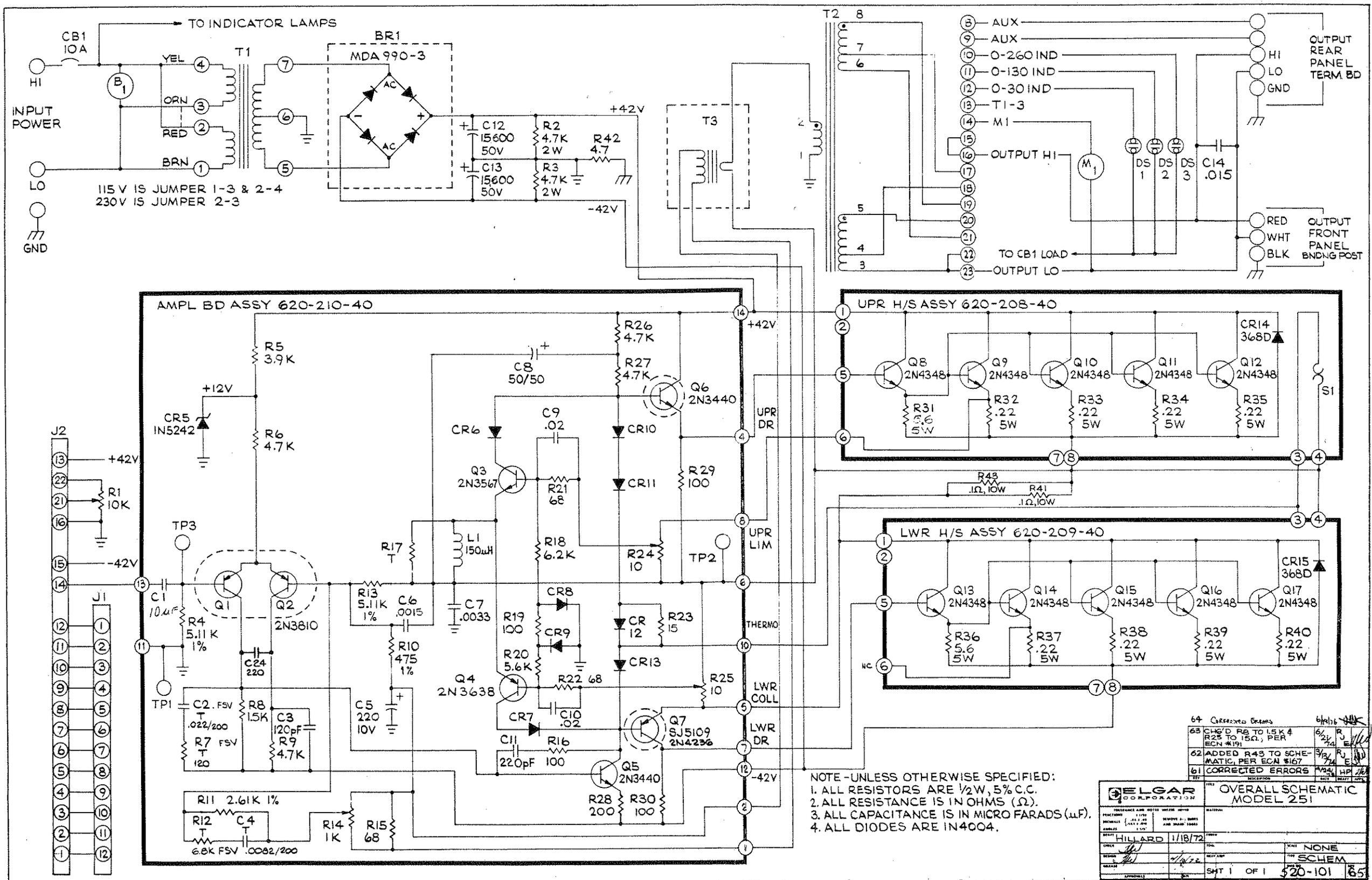
Figure 7-1. Model 251 Overall Schematic, Dwg. No. 520-101-6X
