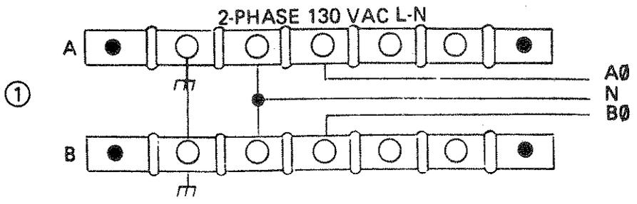
NOTE: 28V OR 230V OUTPUTS ARE ALSO AVAILABLE FOR ALL CONFIGURATIONS EXCEPT 3 AND 5, BY ROTATING VOLTS SELECT CARD TO DESIRED OUTPUT VOLTAGE POSITION
