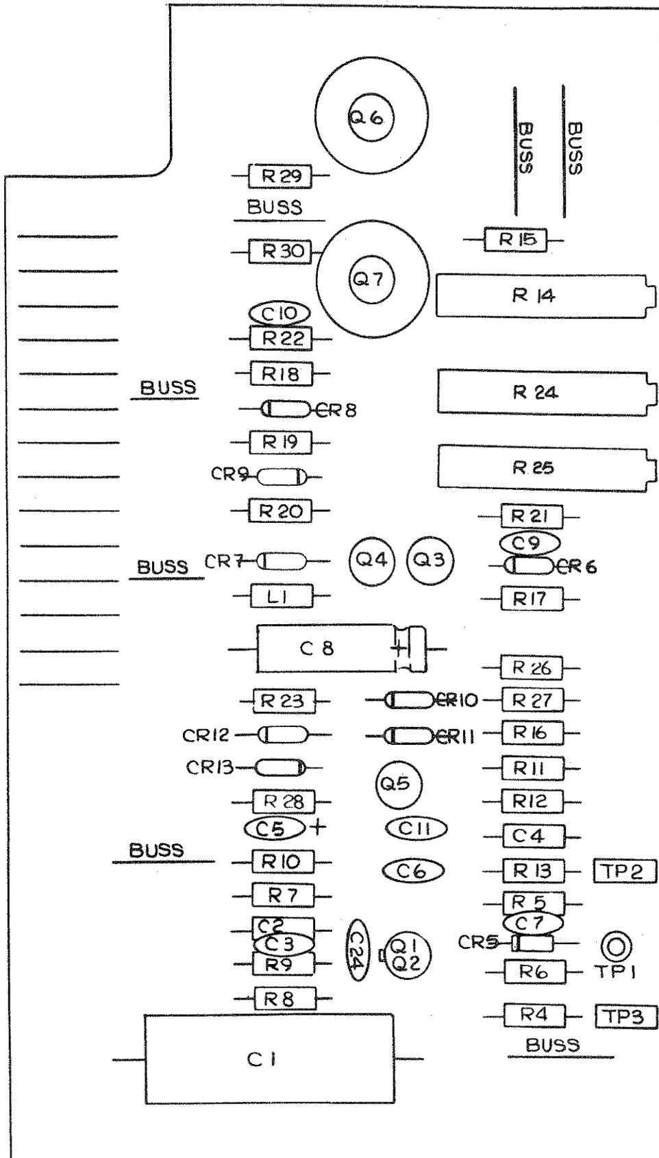
Figure 7-3. Models 251 and 501A Amplifier Board Assembly Parts Layout, Dwg. No. 620-210-00
