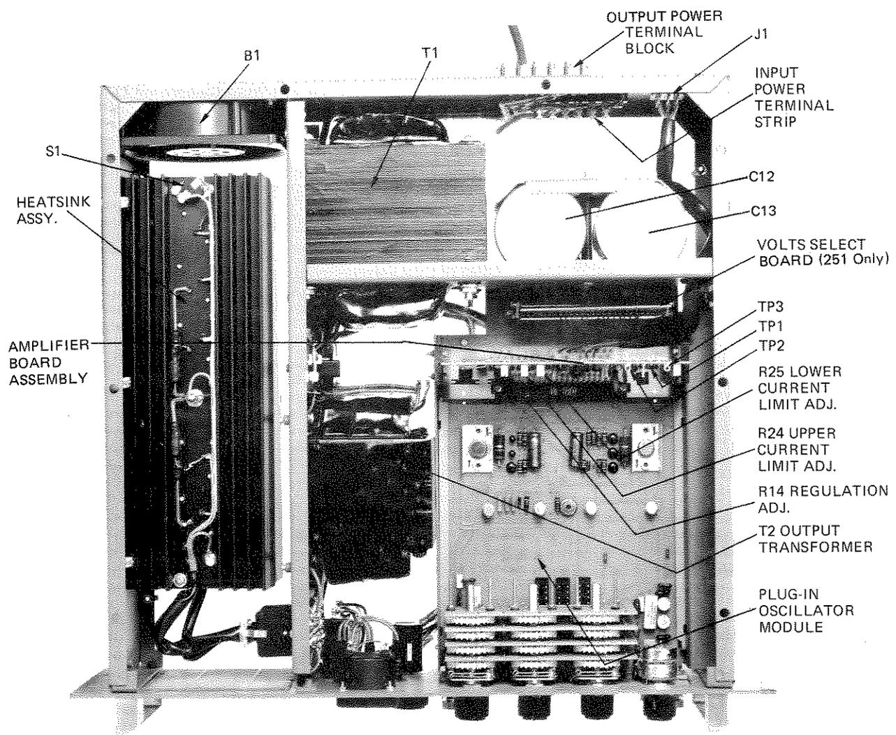
Figure 5-1. Model 251 Top View
